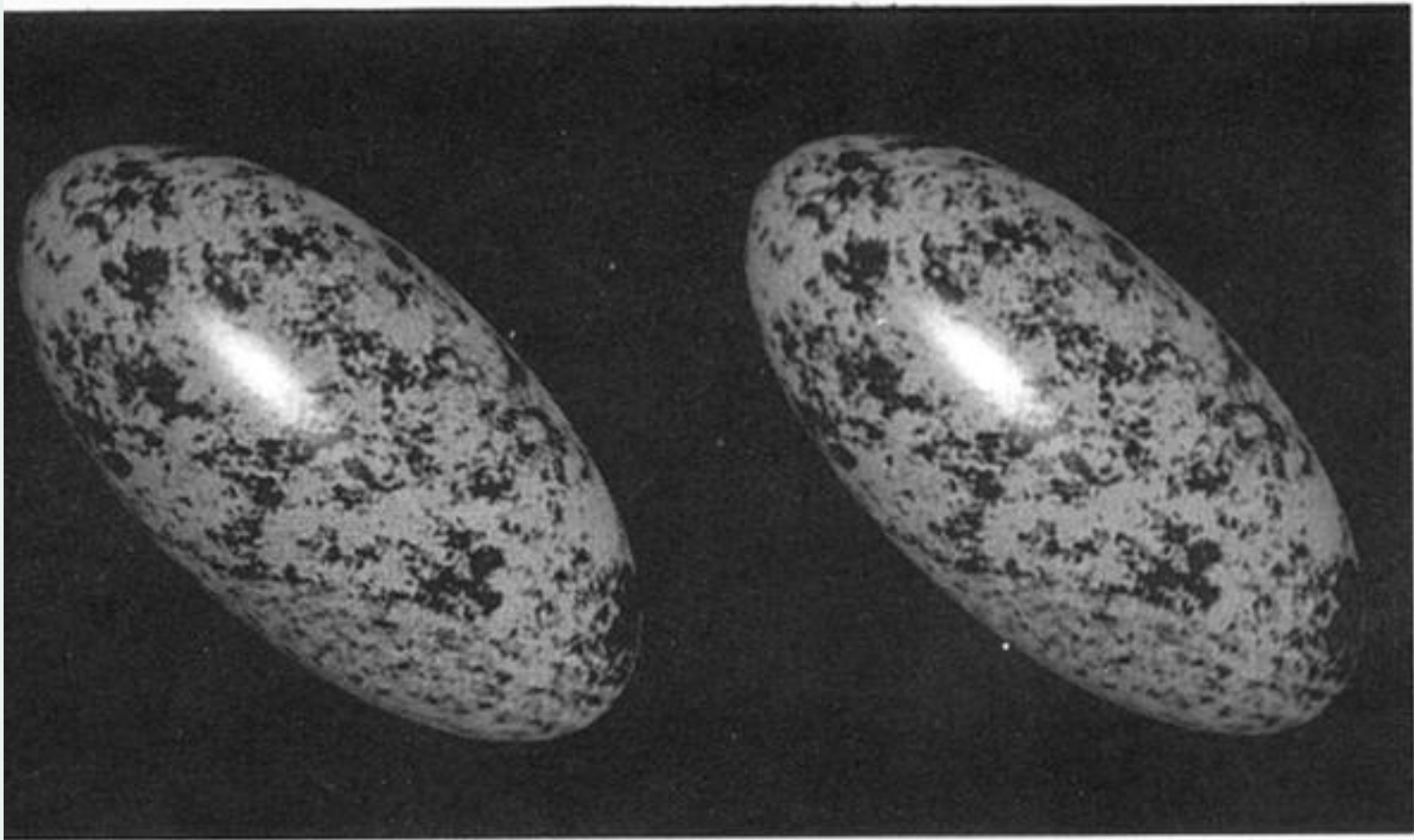
Figure 6. The displacement of the specularity in the right (versus left) image is oblique, whereas that of any nearby surface feature is horizontal. The surface feature is constrained by epipolar geometry but the specularity is not.
